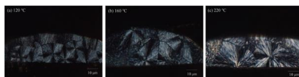
Fig.1 POM image of isothermally melt-crystallized PPS [1]
