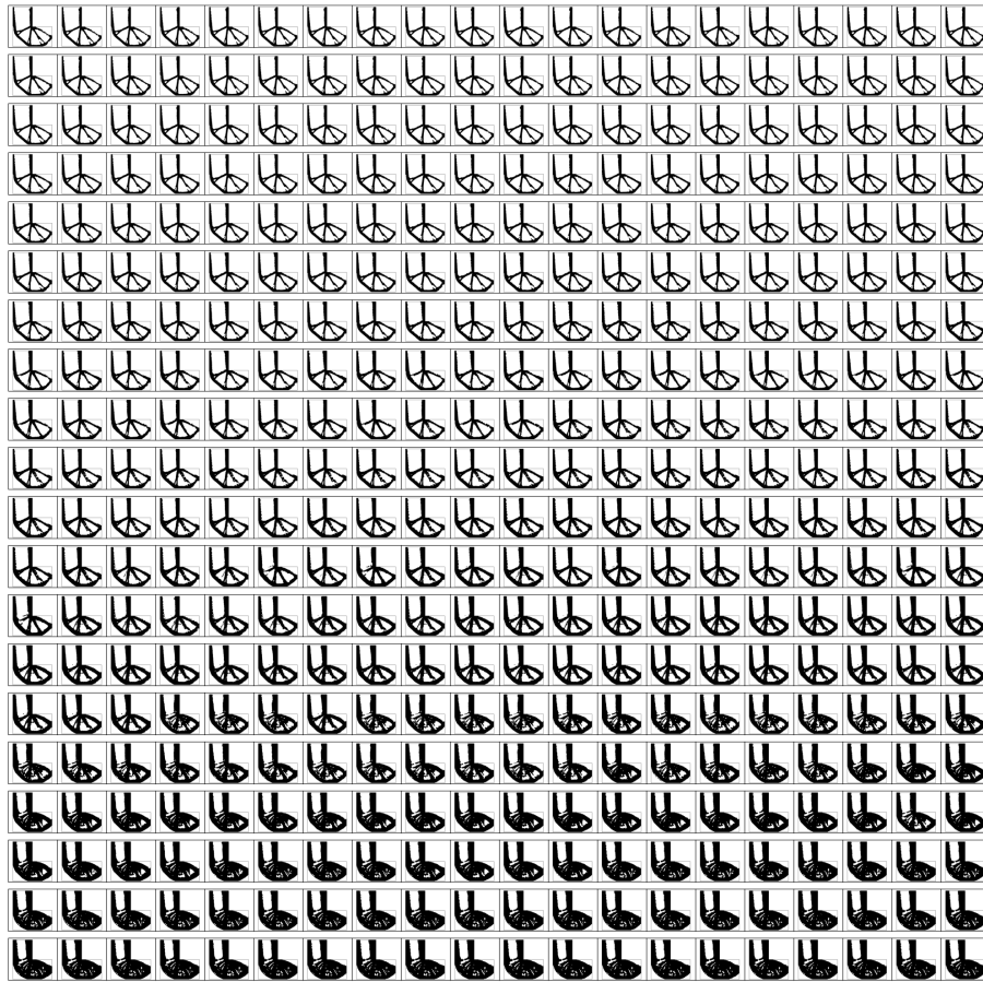
Fig. 9: Material distribution with 262,144 dimensions generated by proposed method of the elite data at iteration 50
