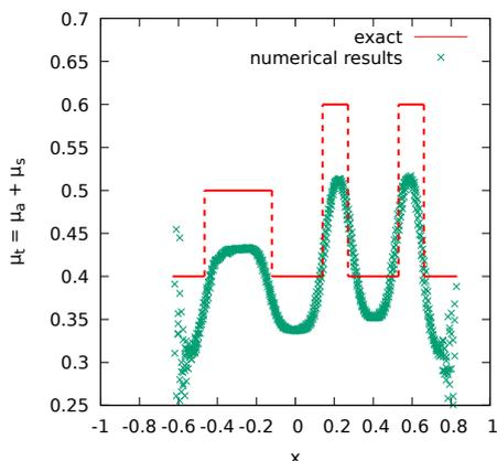
図-4 Green symbols (x) show reconstructed attenuation coefficient  $\mu_t$  on the yellow dotted segment in Fig. 3, while red shows exact value.
