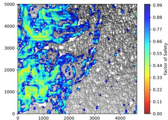
Fig. 4 Distribution of collapse in earthquake condition
