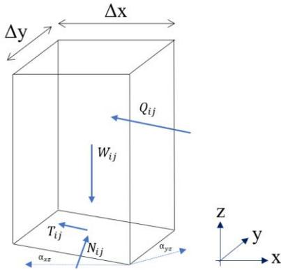
Figure. 1 Force acting on a divided column
