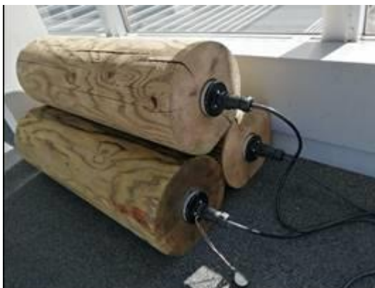
Fig. 2 Off-grid system with log covered batteries
