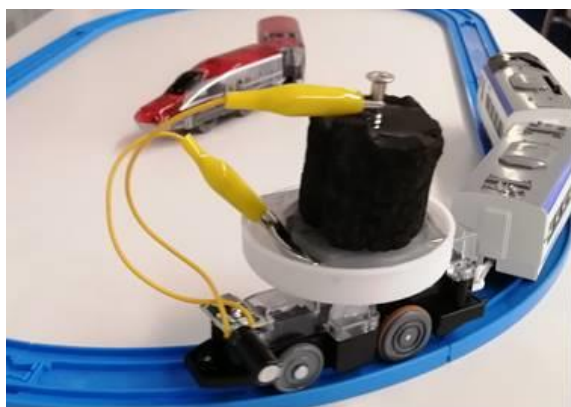
Fig. 1 Electric train powered by Binchotan coal
