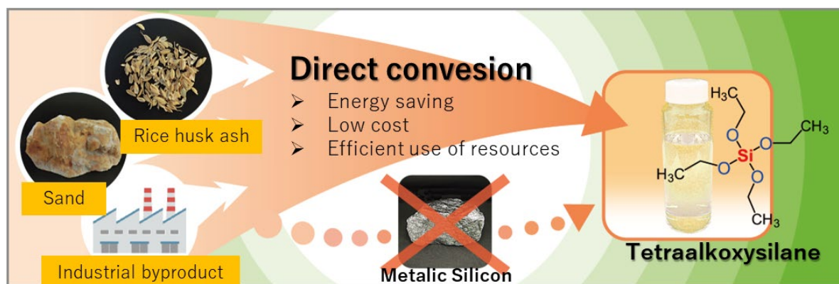
Figure 2. Direct Synthesis of Tetraalkoxysilane from Silica
