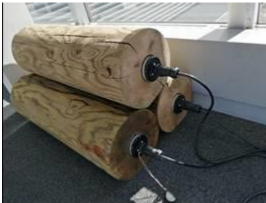
Fig. 2 Off-grid system with log covered batteries
