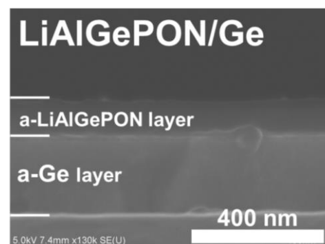
Fig.2 SEM image of LiAlGePON/Ge multilayer anode film
