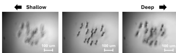
Fig.1 Image of defects in glass substrate
