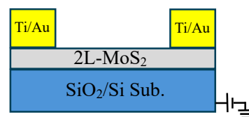
Fig.2 Device structure of MoS 2
