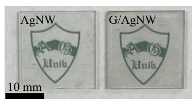
Fig 1. Photograph of AgNW and graphene-AgNW hybrid films on a quartz glass
