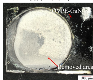
Fig. 1. OVPE-GaN substrate almost removed by etching
