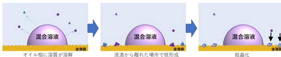
Fig.2 Possible extra-droplet crystallization mechanism
