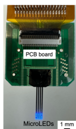
Fig. 1 Photograph of a needle-shaped MicroLED device
