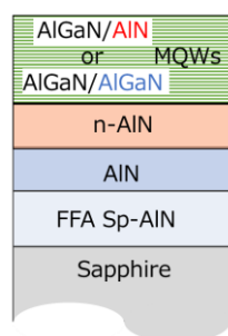
Fig. 1 Schematic image of sample structures of MQWs.
