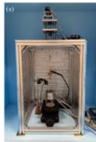
Fig.1 Set-up for the Czochralski growth of triglycerides.
