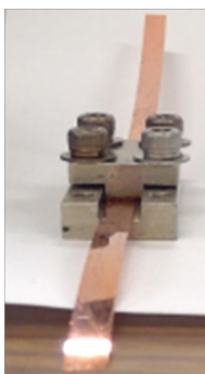
Fig.1 Photograph of REBCO tapes fixed by metal fittings.
