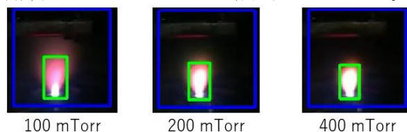
Fig. 1 Images of YBCO ablation plumes at different O 2 pressures.
