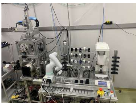
Figure 1: Automated arc-melting system.
