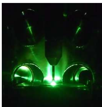
Figure 2: Arc-melting in automatic motion.
