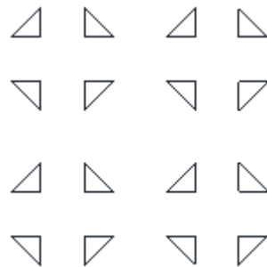
[Figure 1] Figure of the proposed magnonic crystal design with four unit cells.
