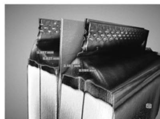
Battery Inspection for Overhang Distances
